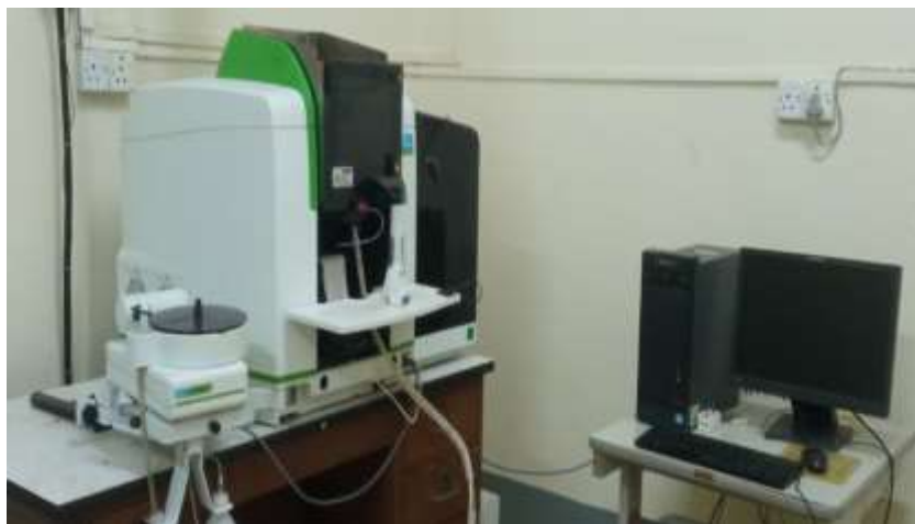
Figure 5. Atomic Absorption Spectroscopy (AAS) (Perkin Elmer AA900H), Universities Research Center, University of Yangon
