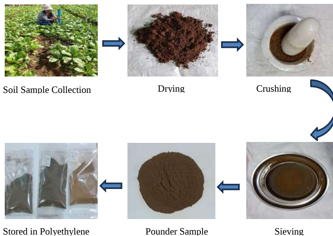
Figure 2. Collection and preparation of soil samples
